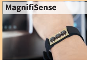
MagnifiSense Wrist-worn magnetic sensor that monitors daily activity
