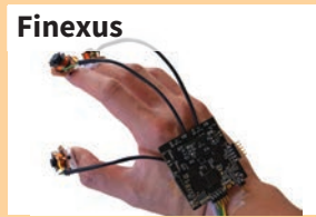
Finexus Tracking accurate finger motions using magnetic sensing
