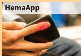
HemaApp Noninvasive screening of hemoglobin concentration using a smartphone camera
