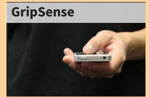
GripSense Using built-in sensors to detect hand posture and pressure on phones
