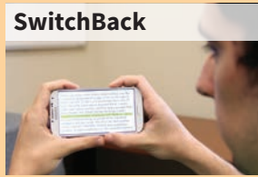
SwitchBack Using gaze tracking on smartphones to guide attention for task resumption
