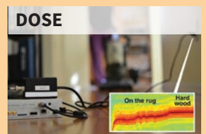
DOSE Sensing operating states of home electronic appliances from EMI
