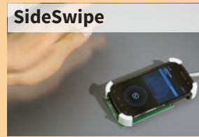
SideSwipe Detect in-air gestures using unmodified GSM signals
