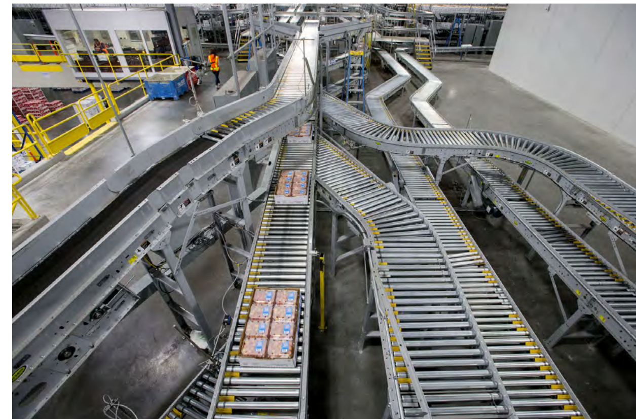
Cherries packed in clam shells move along a conveyor highway to be shipped to destinations around the world at Stemilt Growers’ new shipping facility north of Wenatchee.
